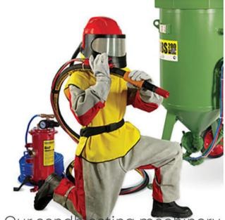
Our sandblasting machinery is designed to effectively remove mill scale, rust, and oil from steel surfaces accumulated during the manufacturing process, offering a cost-effective solution for surface cleaning. We follow the Sa 3 - SSPC-SP 5 standard to ensure thorough surface preparation. The white blast cleaning process uses dry abrasive blasting to eliminate old coatings, rust, flaky mill scale, and other contaminants. preparing the surface for subsequent treatment.
